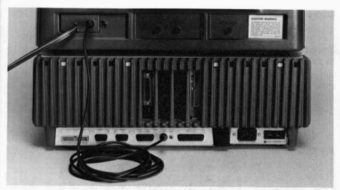
Figure 2-2. Connecting the video monitor
