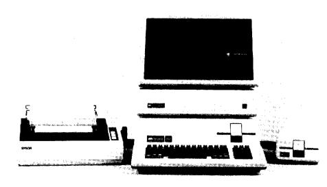
Figure 1-2. Expanded Apple III system
