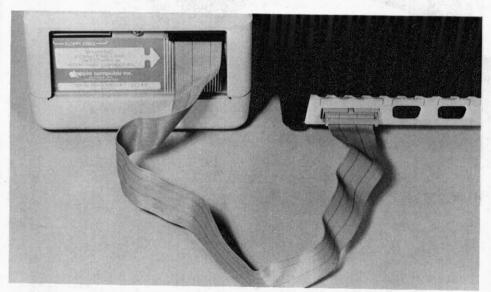
Figure 2-3. Connecting the Apple Disk III
