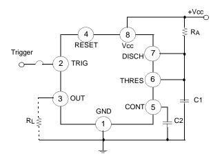
Figure 1. Monoatable Circuit
