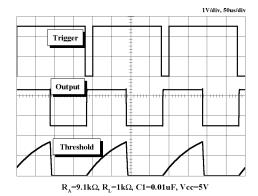
Figure 3. Waveforms of Monostable Operation
