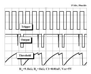
Figure 4. Waveforms of Monostable Operation (abnormal)
