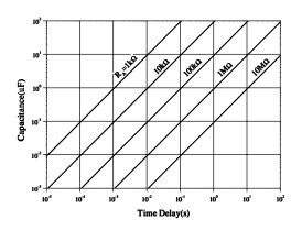
Figure 2. Resistance and Capacitance vs. Time delay(td)
