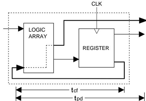
**f<sub>max</sub> with Internal Feedback 1/(tsu+tcf)**
