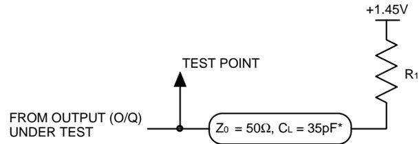
\*C<sub>L</sub> includes test fixture and probe capacitance.
