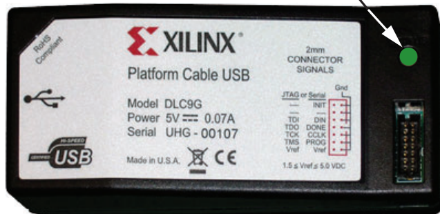
Figure 11: Status LEDs Indicating Target Voltage
