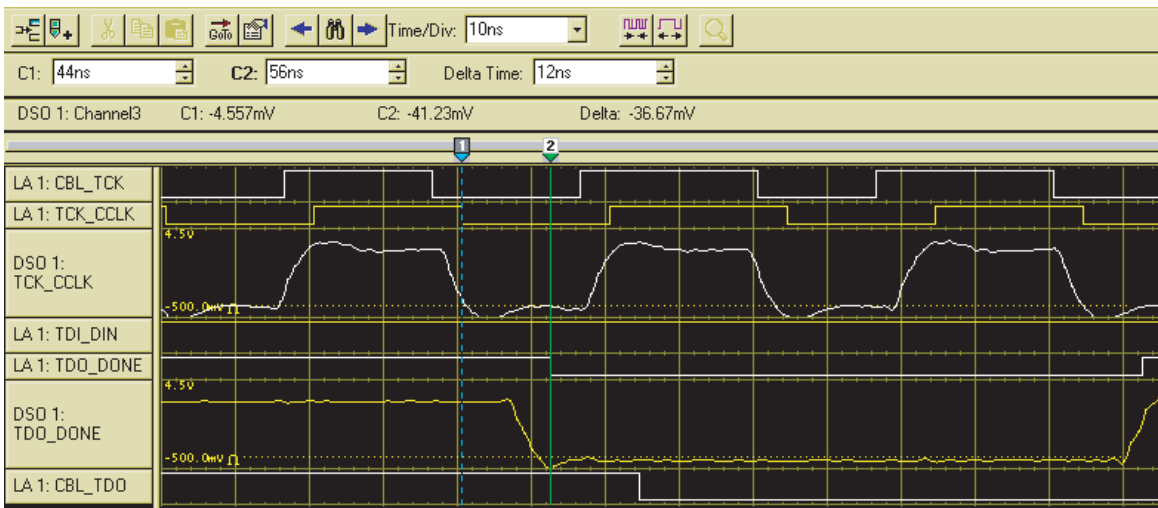
Figure 20: TDO_DONE_MISO Timing with Respect to TCK_CCLK_SCK (TCK_CCLK_SCK to TDO_DONE_MISO Delay)
