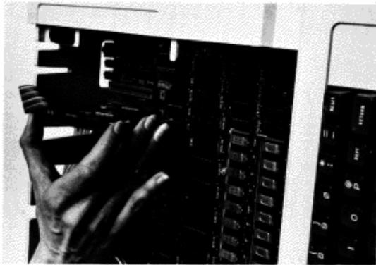
Inserting the Controller Card
